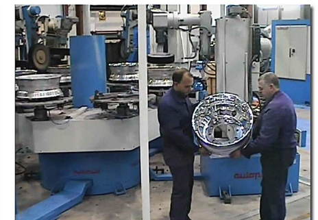
5 CNC head rotary transfer polishing machine with 26 interpolated axes for internal polishing of aluminium alloy truck wheels.
