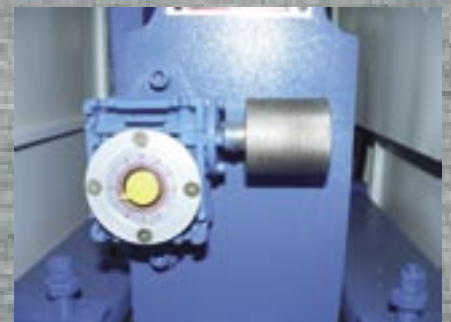
Adjustable Contact Drum for use with Scotch Brite Belts
