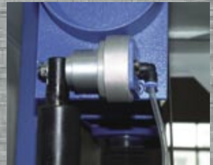
Patented Pneumatic Controlled Abrasive Belt Tracking
