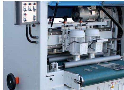
Height adjustment by handwheel or motorized (option)
